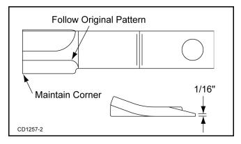
Figure 14. Blade Sharpening
